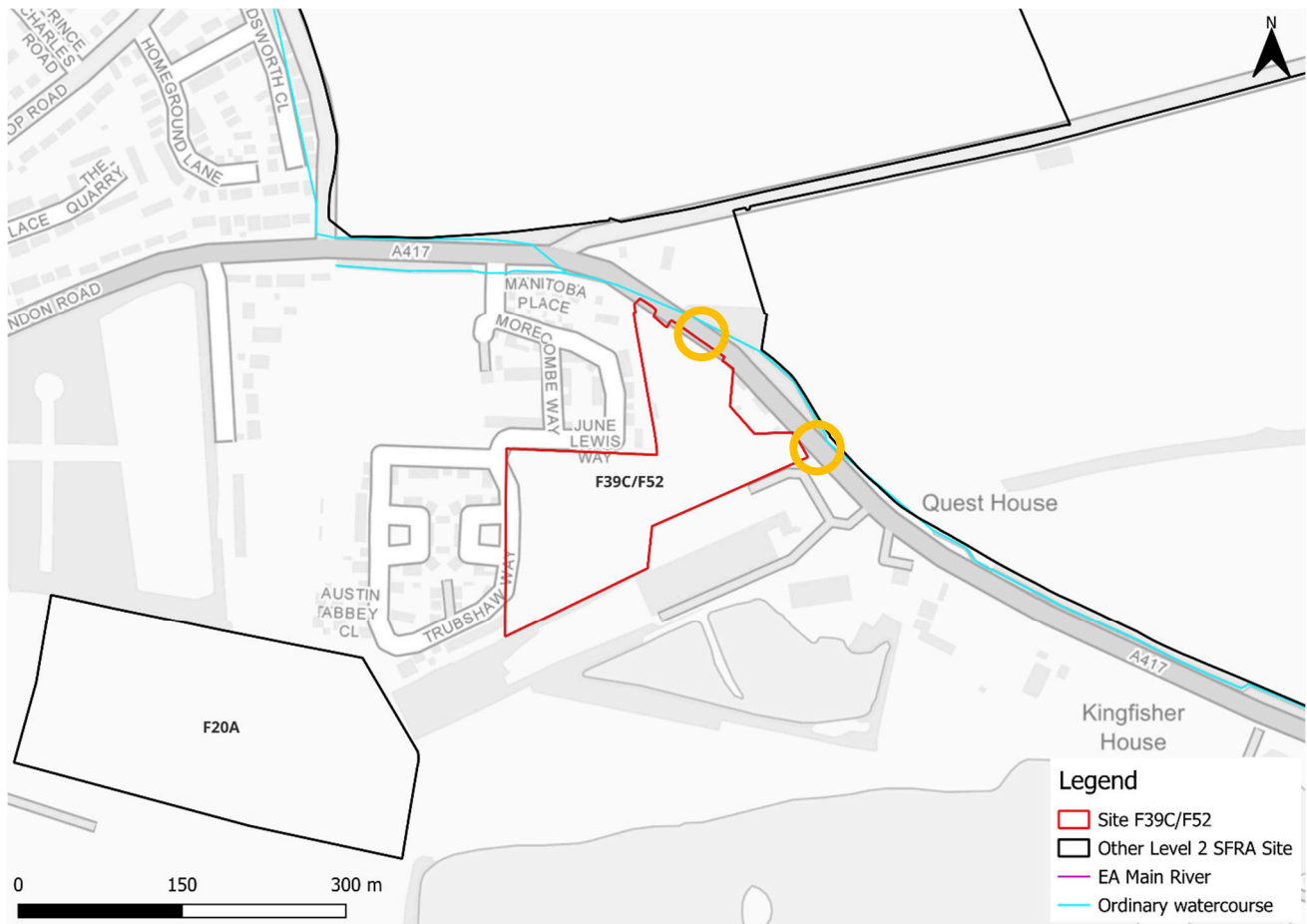
Figure 2-3: Potential access and escape routes
