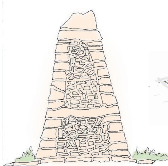
Figure 43: Example showing the construction of dry-stone wall.
