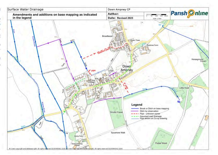
Figure 5.4 Surface Water Drainage Detail
